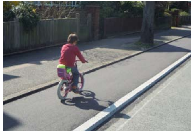
Split-level kerbs provide light segregation
