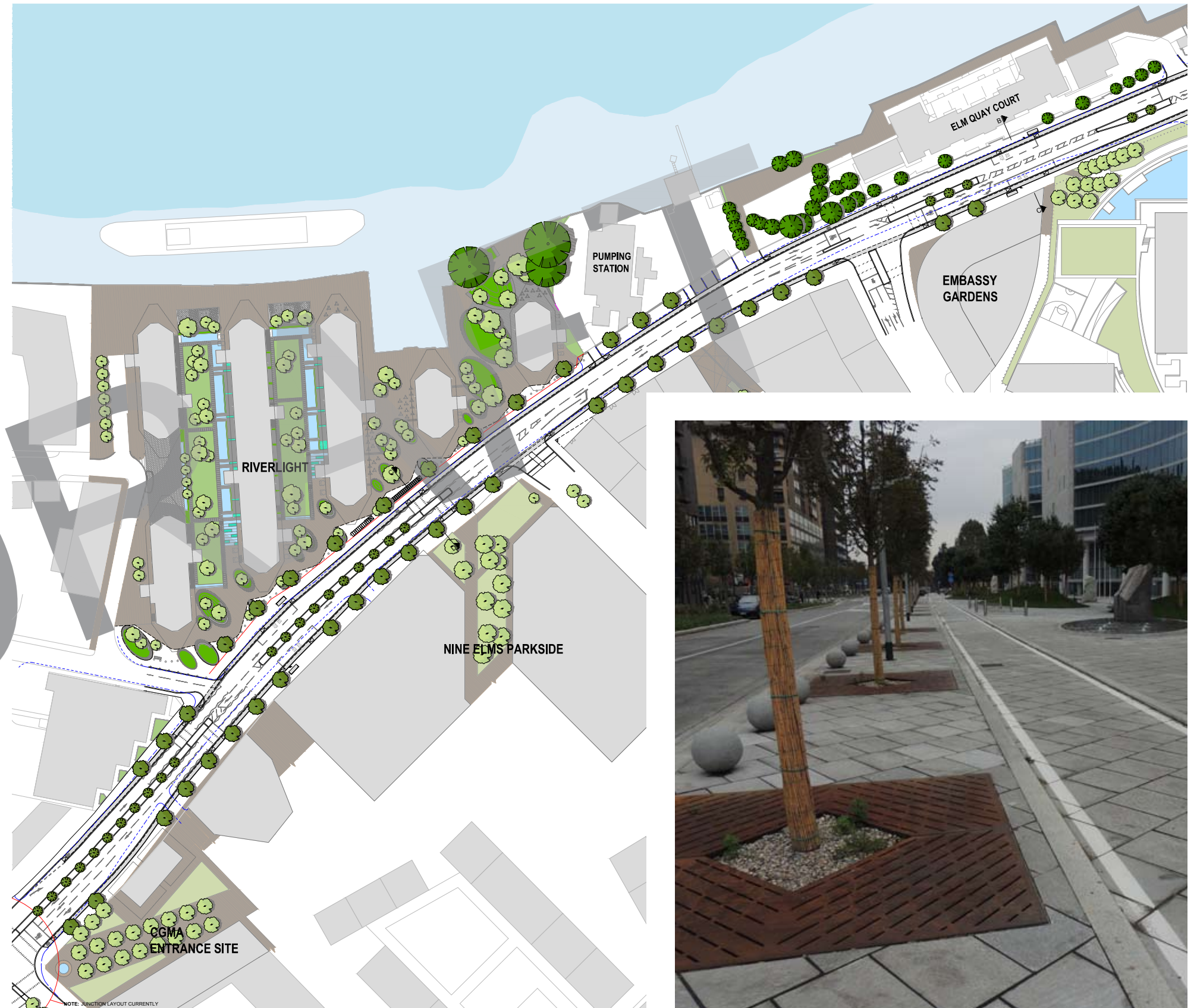
Draft plan for full-length segregated cycle tracks along Nine Elms Lane (Burns + Nice)
